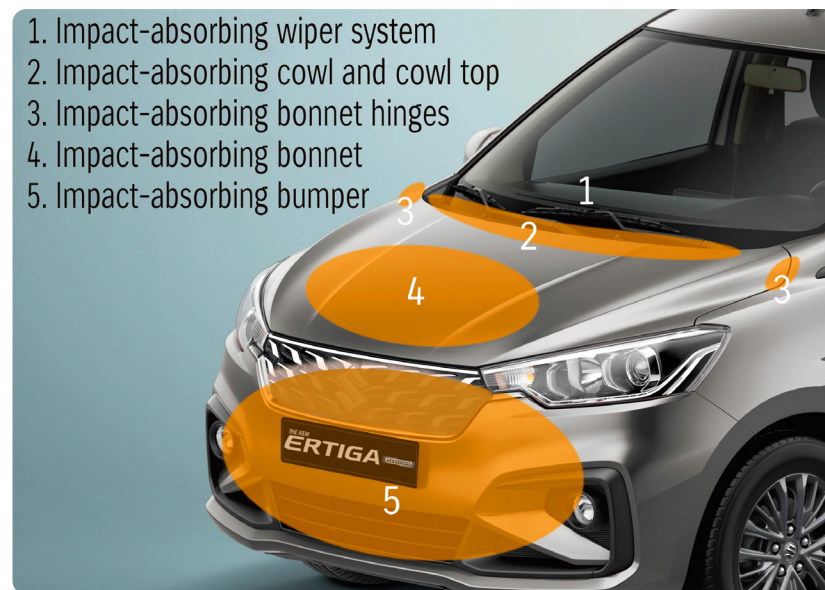
Pedestrian injury mitigating body Helps mitigate head and leg injury in the event of a collision with Pedestrian
