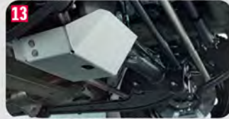
13 FRONT DIFFERENTIAL GEAR GUARD Part No.: 9912J-78R31-000 MADE OF 3mm ALUMINUM PLATE.
