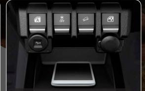
USB AND ACCESSORY SOCKETS A 12V accessory socket, and a USB socket to allow connection to the audio system.
