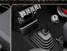
The manual transmission system has optimized gear ratio that offers fuel efficiency. The shift lever is designed to reduce vibration and has a direct shift
