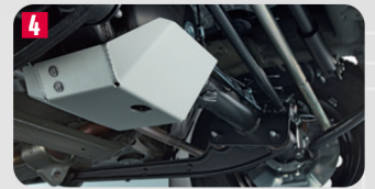
4 FRONT DIFFERENTIAL GEAR GUARD Part No.: 9912J-78R31-000 MADE OF 3mm ALUMINUM PLATE.
