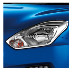
Headlamps (Halogen multi-reflector)
